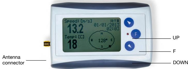
**Receive data** LED blinks every time when new data are received– every 2 seconds at normal reception. In case the display unit has no data from sensor for 30 seconds it shows two dashes. Signal strength is numerically shown in dB.
